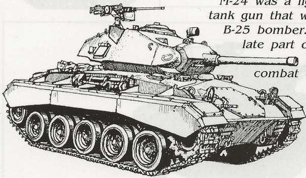
M-24 was a light tank mounting a 75mm tank gun that was originally developed for B-25 bomber. Debuted and deployed in late part of WWII. Later, M24 encountered its real combat during the Korean War.
