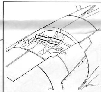
Please note: The model cannot rest on its wheels with the airbrake in the fully open position.
