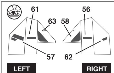
NOTE: APPLY DECALS ON INSIDE SURFACES OF INTAKE ASSEMBLIES AS SHOWN.
