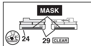
NOTE: MASK BOTH SIDES OF PART # 29 AS SHOWN BEFORE PAINTING. REMOVE MASK AND APPLY DECAL TO INSIDE OF DOOR SO IT WILL BE SEEN FROM BOTH SIDES.
